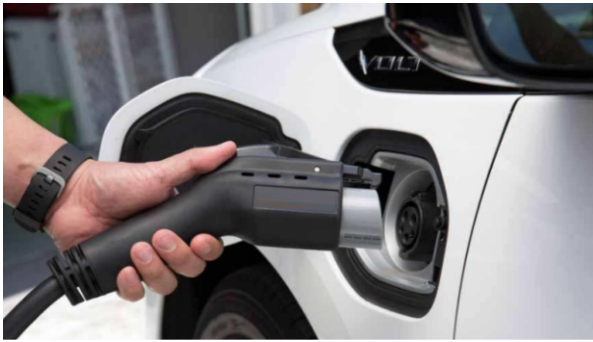
Step 1: Plug in the charging connector
